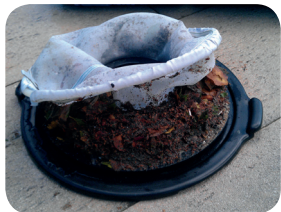
Filtering options 105, 250 or 1000 microns filter bag
