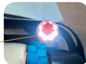
With 2 infra red sensors, tilt sensor
